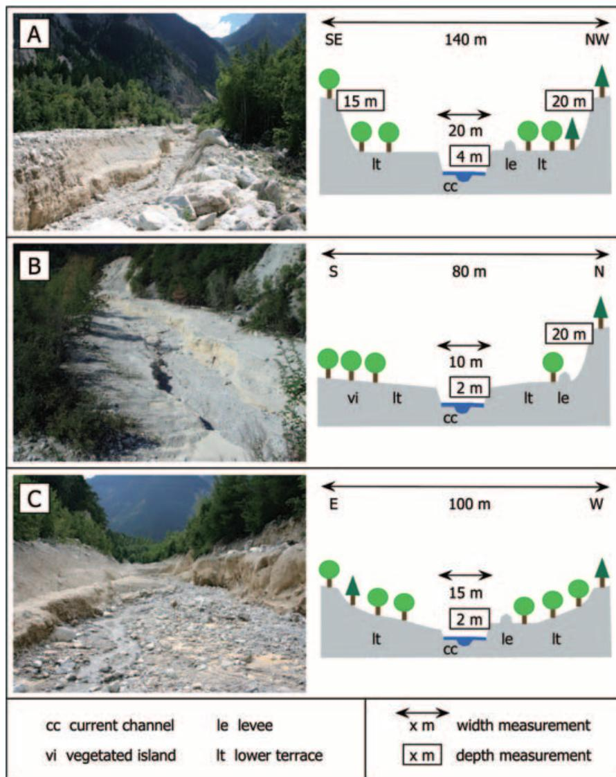
**Figure 2.** Views and cross-sections of the current channel and lower terraces at the three investigated sectors. In sector 1 (A), the channel is deeply incised. By contrast, the Illgraben has formed a much less incised channel in sector 2 (B) and in sector 3 (C). This figure is available in colour online at [www.interscience.wiley.com/journal/espl](http://www.interscience.wiley.com/journal/espl)
