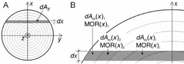
Figure A1. (A) Log cross section with schematic, enlarged annual year rings. Axes:  $z$  is the height above the stem base, and  $y$  the axis of applied bending moment in the tests, which causes deflections in the  $x$ -direction. (B) Enlargement of the upper left part of (A). Modulus of rupture (MOR) of each area element  $dA_y$  is calculated (Equation 15) on the basis of  $\text{MOR}(x)_i$  of finite area elements  $dA_{xy}(x)_i$ .
