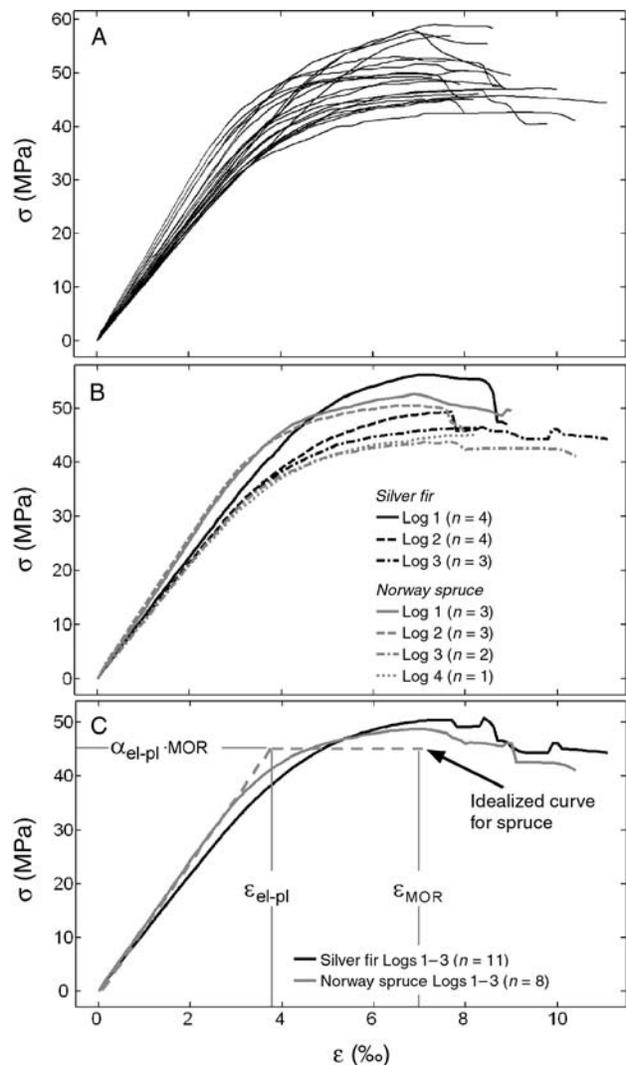
Figure 2. (A) Bending stress ( $\sigma$ ) as a function of bending strain ( $\epsilon$ ) for all 20 logs from silver fir (*Abies alba*) and Norway spruce (*Picea abies*) trees. Mean  $\sigma(\epsilon)$  for logs grouped by (B) height and species and (C) by species. The idealized stress–strain curve in (C) is ideally elastic up to a percentage  $\alpha_{el-pl}$  of the modulus of rupture (MOR), and ideally plastic between  $\epsilon_{el-pl}$  and  $\epsilon_{MOR}$ .
