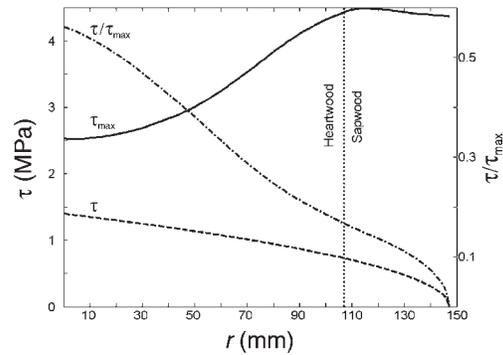
Figure 4. Shear stress ( $\tau$ ), shear resistance ( $\tau_{max}$ ) and their ratio as functions of radial distance from pith ( $r$ ) in logs of silver fir (*Abies alba*) and Norway spruce (*Picea abies*) trees. Means are shown for all logs as MOR was reached and for the stem cross section where the highest ratios were found (below location of force application at the thinner side of the log). Shear failure occurred in the outer heartwood, i.e., about  $60 < r < 100$  mm.
