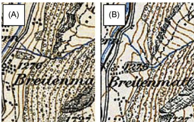
Fig. 5. Germination dates of the sampled trees suggest that a devastating debris-flow event in the 1880s had cleared the surface and scoured the currently active channel. This interpretation is supported by topographical maps from 1881 to 1891, which show a dislocation of the channel (Swisstopo, 2006).
