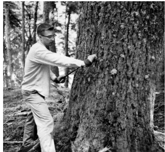
Figure 2. R.S. Sigafoos in the field employing an increment borer in order to date past geomorphic events. Credit: US Geological Survey, Department of the Interior, US Geological Survey.
