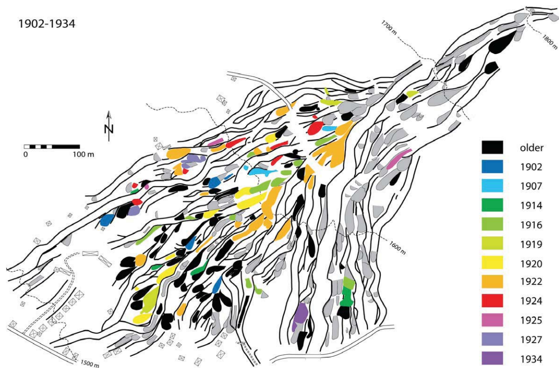
Figure 8. Deposition of debris-flow material on the cone of the Ritigraben torrent between 1902 and 1934. Only events associated with >600 \text{ m}^3 on the present-day surface of the cone are indicated on the map. Deposits shown in black are dated, but are older than the time segment illustrated.
