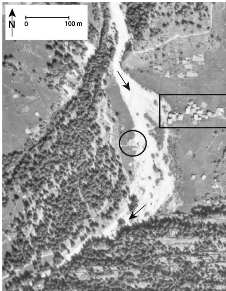
Fig. 9. Aerial photograph of the Bruchji cone taken in May 1936. Two buildings (circle) are located within the deposits and appear to have been severely affected by the debris-flow event reconstructed for 1935. Towards the northeast of the damaged building, houses of a small hamlet (rectangle) are found very close to the deposition zone of the 1935 event as well. Arrows indicate the flow direction of water in the torrent (aerial photograph reproduced with courtesy of swisstopo (BA068080)).
