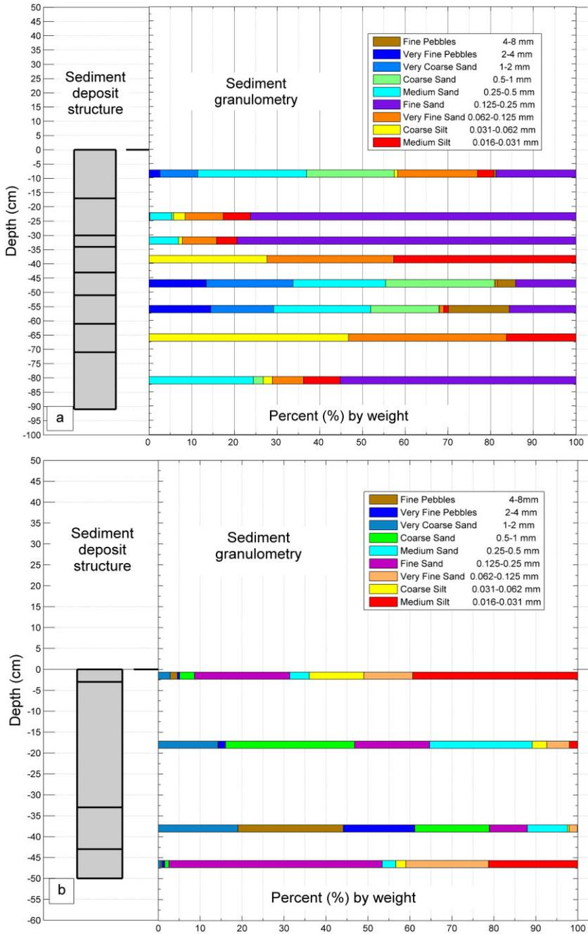
Fig. 5. (a-c) Granulometric characteristics of the sediment deposits.
