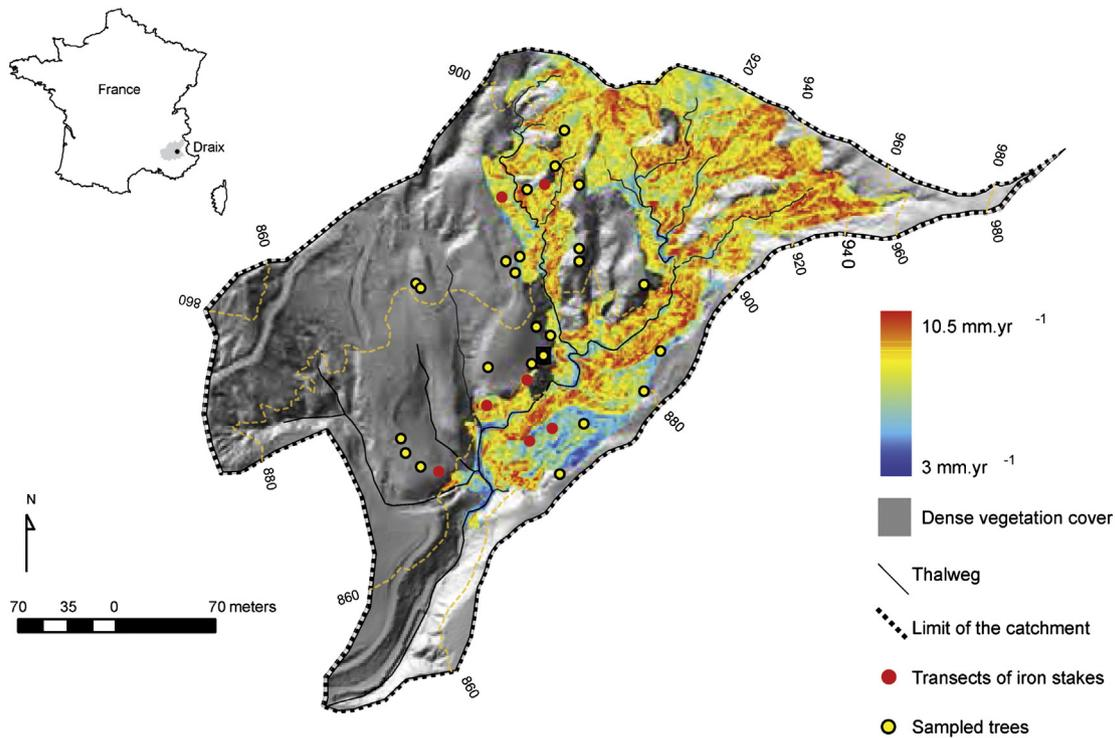
**Fig. 4.** High-resolution erosion maps for the Laval catchment, Draix experimental basin, southern French Alps. Predicted erosion maps are obtained through a coupling of (i) the linear regression model obtained from dendrogeomorphic erosion rates from *Pinus sylvestris* roots (yellow dots) with (ii) high-resolution slope maps of the Laval catchment derived from a LiDAR-generated DEM.
