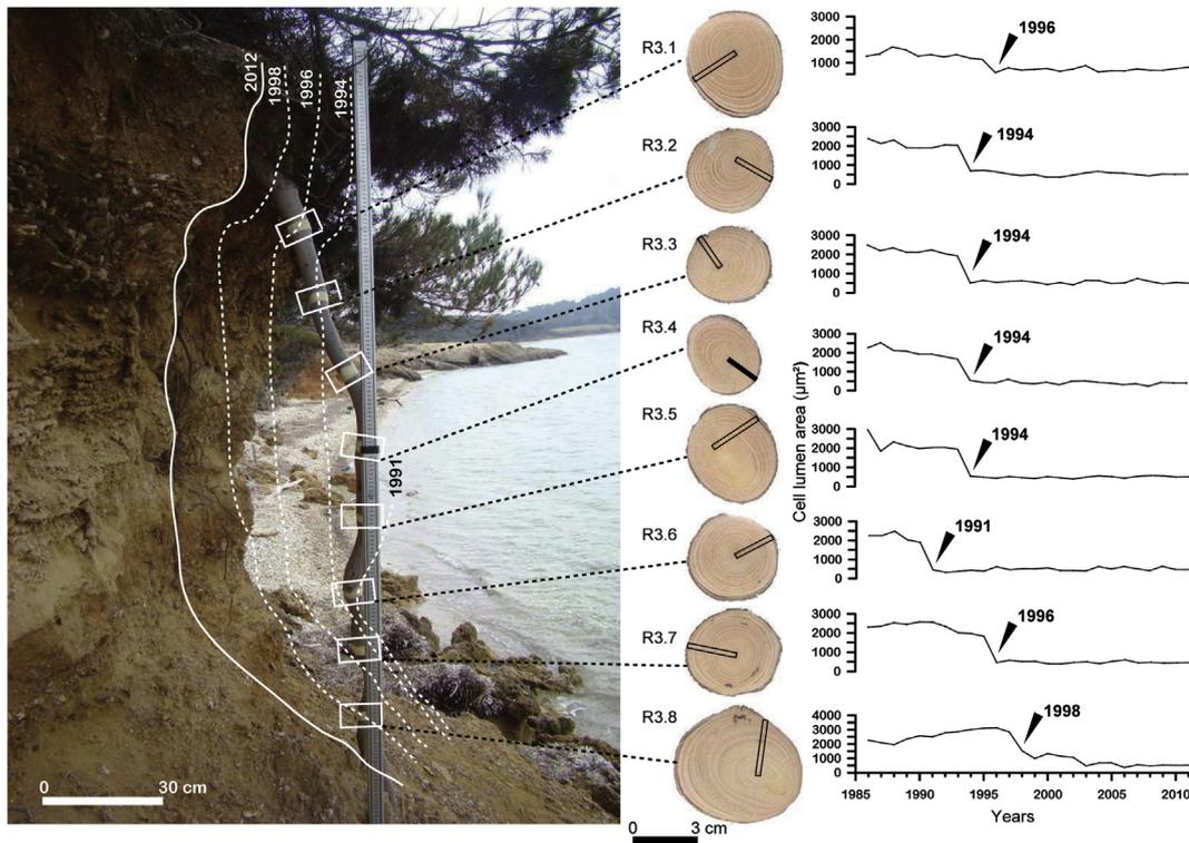
**Fig. 8.** Reconstructed rates of cliff erosion derived from exposed *Pinus halepensis* roots hanging from decametric, detritic cliffs of Porquerolles Island (Var, France). The analysis of oblique roots also allows analysis of temporal changes in cliff profiles, and thus could become a valuable tool for the assessment of the temporal frequency or changes in storminess.
