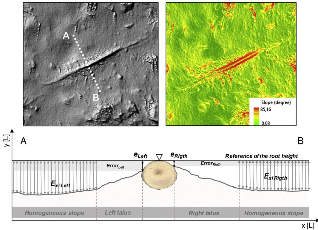
**Fig. 11.** High-resolution TLS-derived DEM of a sandy badland environment with an exposed root and illustration of the impact of the root on micro-topography and transversal soil profiles on both sides of the root. This effect only disappears at some distance from the root, the height of the exposed part of the root ( $E_x$ ) should not be measured at the point where the root converges with the soil.
