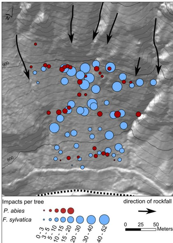
**Fig. 3.** Absolute numbers of impacts on individual trees at Hechenberg. Although *F. sylvatica* shows much more evidence of rockfall activity as compared to *P. abies*, the distribution of zones strongly and less affected are comparable.
