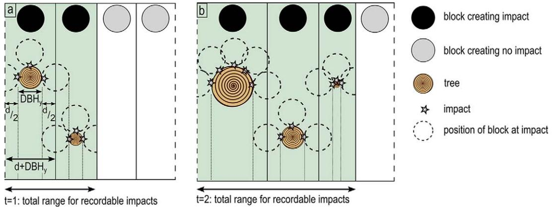
**Figure 2.** Range concept used for the definition of rockfall impact probability in a specific year.
