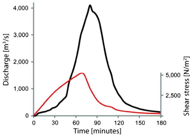
Fig. 6. Outflow hydrograph (black line) and bottom shear stress (red line) over the period of lake outflow as modeled by BASEMENT.
