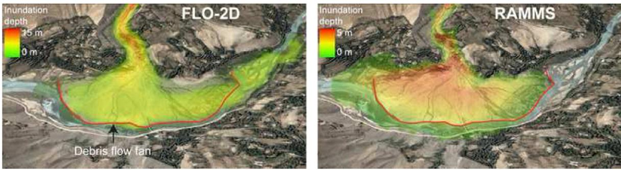
Fig. 12. FLO-2D and RAMMS model calibration and validation based on the 2002 GLOF in Dasht, Tajikistan. Both models produce a debris flow pattern (red line) similar to the real one.
