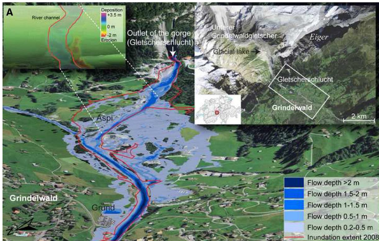
**Fig. 11.** Results of flood and sediment transport modeling of a GLOF at Grindelwald, Switzerland, in May 2008 using BASEMENT. Modeled flooded areas are shown in blue; the actual inundation extent is delineated by the red line. Modeled deposition and erosion are illustrated in the inset. Data from BVE (OIK I), BAFU and swisstopo.
