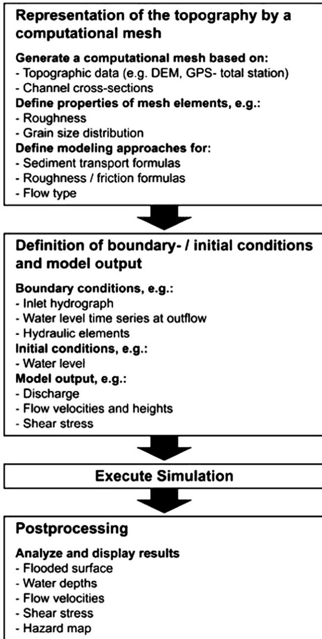
Fig. 2. Typical work flow for dynamic modeling of extreme flow events and related processes.
