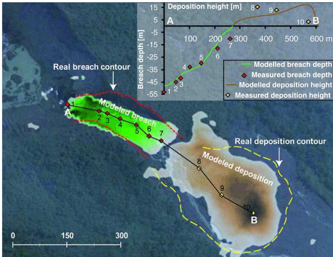
**Fig. 8.** Validation of model results based on a comparison of measured and modeled breach and deposit geometries. BASEMENT calculated breach depths and extent (green), and the depths and extent of outburst flood deposits (brown) that were similar to those observed in the field.
