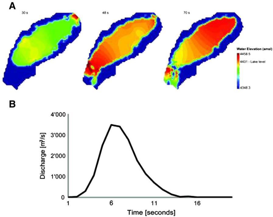
**Fig. 4.** (A) Results of impact wave modeling by IBER at the end of the impact (30 s), at the maximum of the dam overtopping wave (48 s), and after overtopping has finished (70 s). The avalanche impact is from top right, and the colors refer to absolute lake levels above sea level. (B) The outburst hydrograph on the top of the dam, as modeled by IBER.
