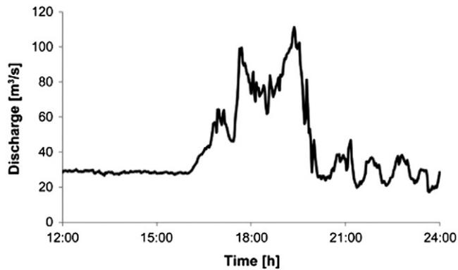
**Fig. 10.** Measured discharge at the outlet of Gletscherschlucht on 30 May 2008 during the GLOF at Grindelwald. Two peaks of  $100 \text{ m}^3/\text{s}$  and  $111 \text{ m}^3/\text{s}$  were separated by 100 min. Data from BVE OIK I.
