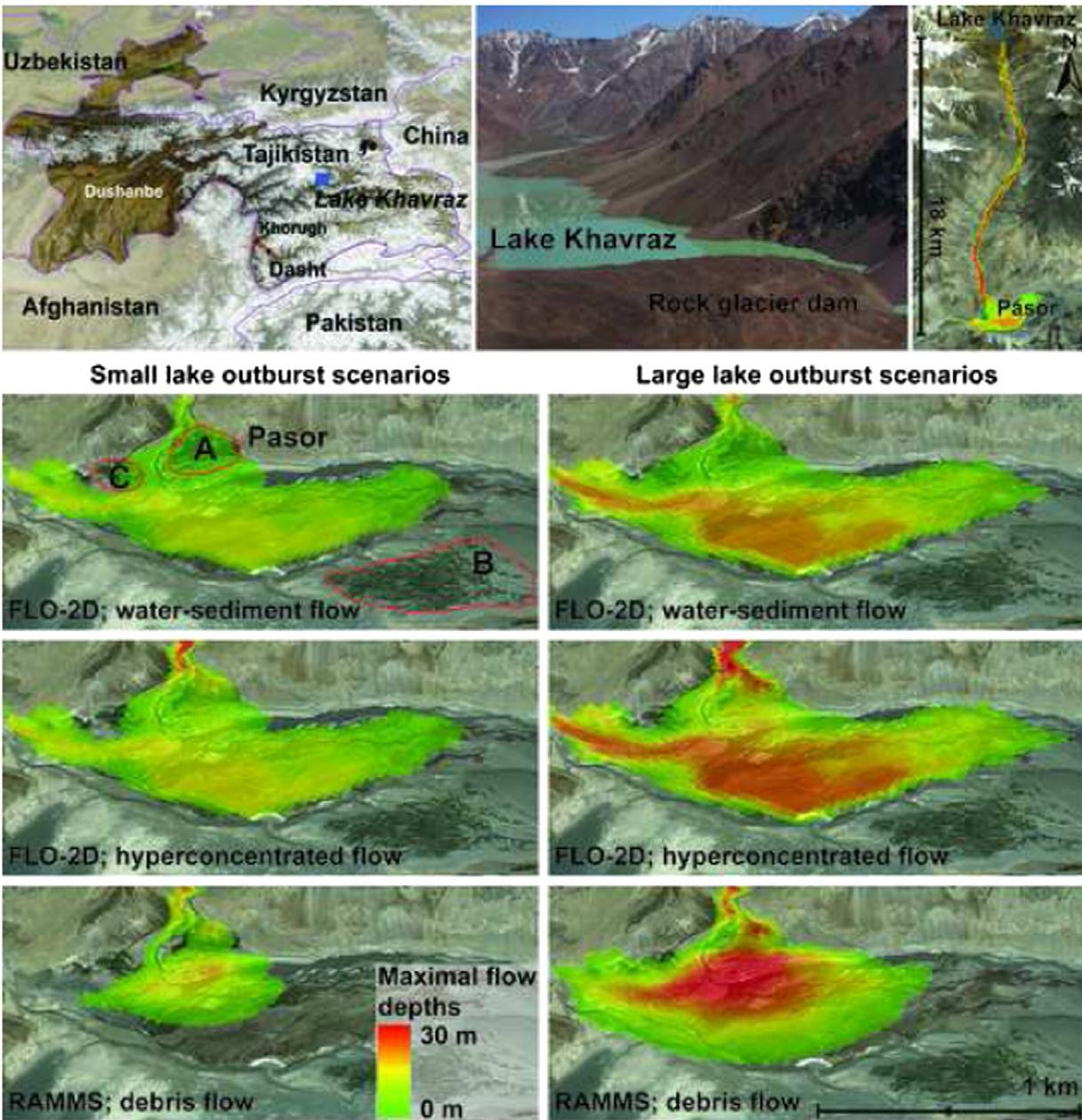
Fig. 13. Scenario modeling of potential lake outburst floods from Lake Khavraz, Tajikistan, using FLO-2D and RAMMS. Different lake outburst scenarios and flow types were modeled. RAMMS results provided by Demian Schneider. Photograph is from TajHaz; satellite images from Google Earth and NASA.
