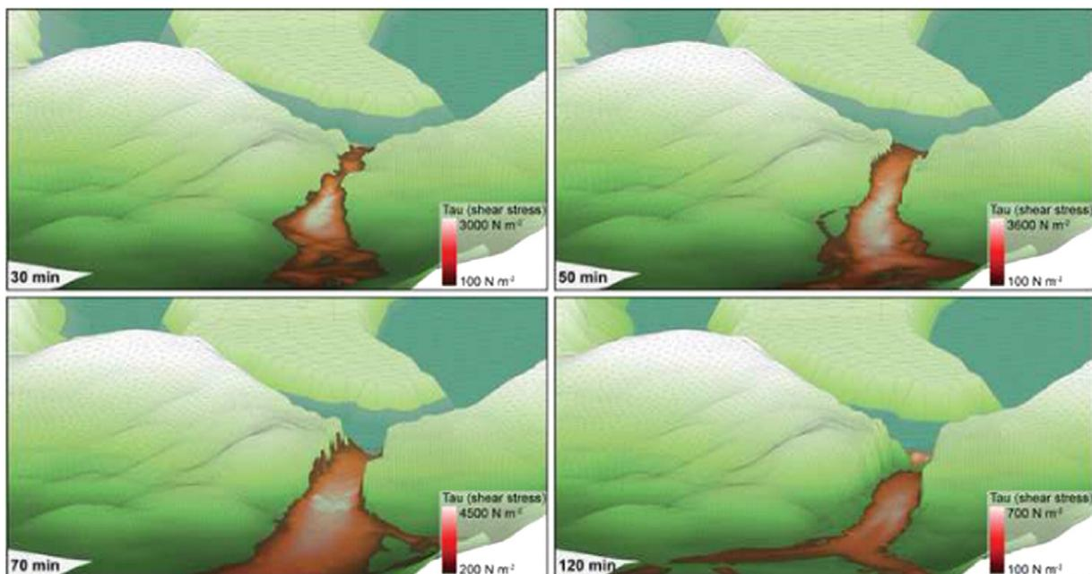
Fig. 7. Dam breach simulation at Ventisquero Negro glacial lake using BASEMENT. The schematic shows the temporal evolution of the breach and bottom shear stress evolution at 30, 50, 70, and 120 min.
