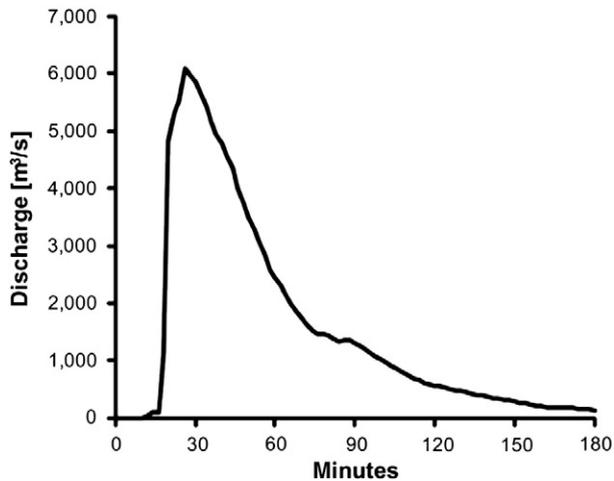
Fig. 16. Hydrograph of the Shako Cho glacial lake outburst calculated by BASEMENT.
