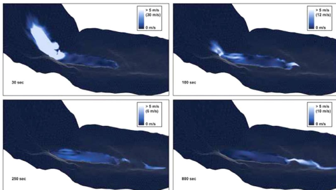
**Fig. 15.** Example of results of impulse wave modeling of Shako Cho glacial lake with BASEMENT. A landslide impact produced waves that overtopped and breached the moraine dam. The four panels show flood velocities (values in brackets are maximum velocities).
