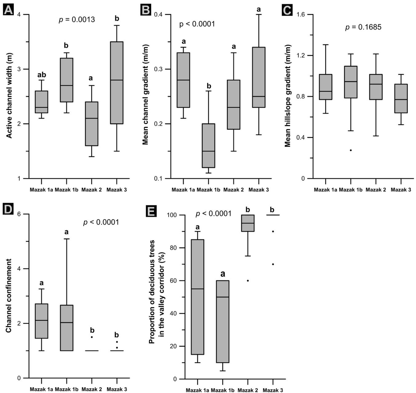
Fig. 2. Boxplots of morphological variables as measured for 20-m long channel reaches in all streams analysed. *p* values provide results of the Kruskal-Wallis test (i.e. active channel width, mean channel and hillslope gradient, channel confinement index and the proportion of deciduous trees in the valley corridor), whereas letters above the boxes point to significantly differing groups (related to post-hoc tests).
